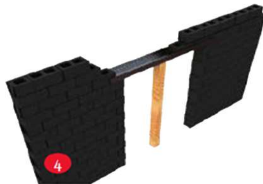
Before laying the blocks down on lintel, place a temporary support beneath the lintel to provide support and to prevent deflection. Temporary support can be removed after the mortar sets, (approximately in 3 to 5 hours).
