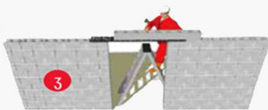
Continuation of block work Can be carried out immediately
